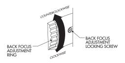
Figure 5. Back Focus Adjustment
